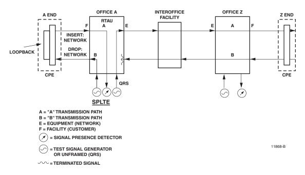
Figure 570-10. Typical End Test Configuration
